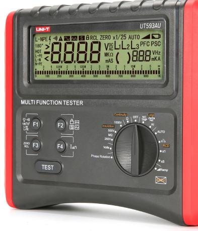
UT593AU is a multifunction digital safety testing instrument, designed with a combination of large-scale integrated analog & digital circuits and the microprocessor chip. It measures RCD, line/loop impedance, continuity, insulation resistance, DC and AC voltage, phase sequence, featuring versatile functionality and high accuracy.
