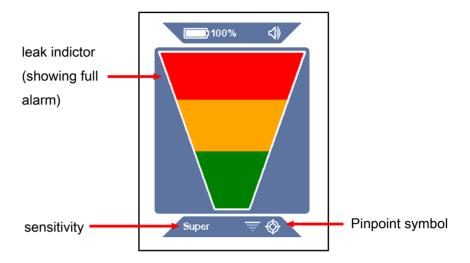
**Pinpoint** mode is identified by a large leak indicator on the display and a **Pinpoint** symbol on the bottom bar. The current sensitivity is also indicated on the bottom bar. This mode works like a standard leak detector with auto-zeroing, where the indicator bars illuminate to indicate when a leak is detected.
