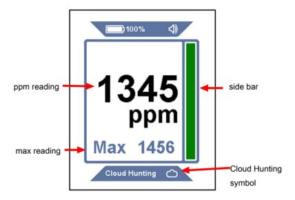
**Cloud Hunting** mode is identified by a large ppm reading on the display and the words **Cloud Hunting** on the bottom, along with a cloud symbol. The side bar increases and decreases with changes in the ppm reading.
